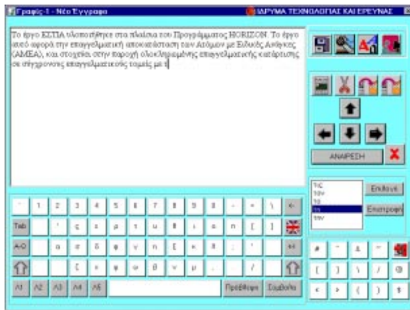
Figure 3: An instance of the word processor GRAFIS for users with motor impairment in their upper limbs
